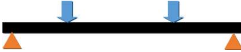
Fig 2: Beam under two point loading
